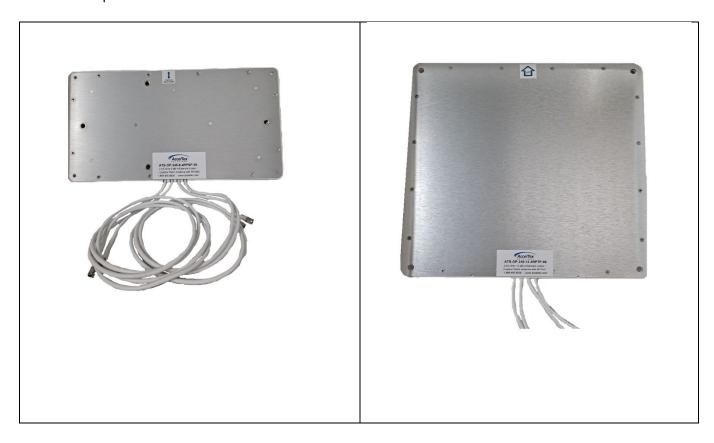
It can be noted that the wider beamwidth of the 13dBi warehouse antenna is on its vertical plane. Where on the 8dBi warehouse antenna, the wider beamwidth is on its horizontal plane. These are the respective planes you want to be aligned with the length of your warehouse aisle to attain full coverage.
