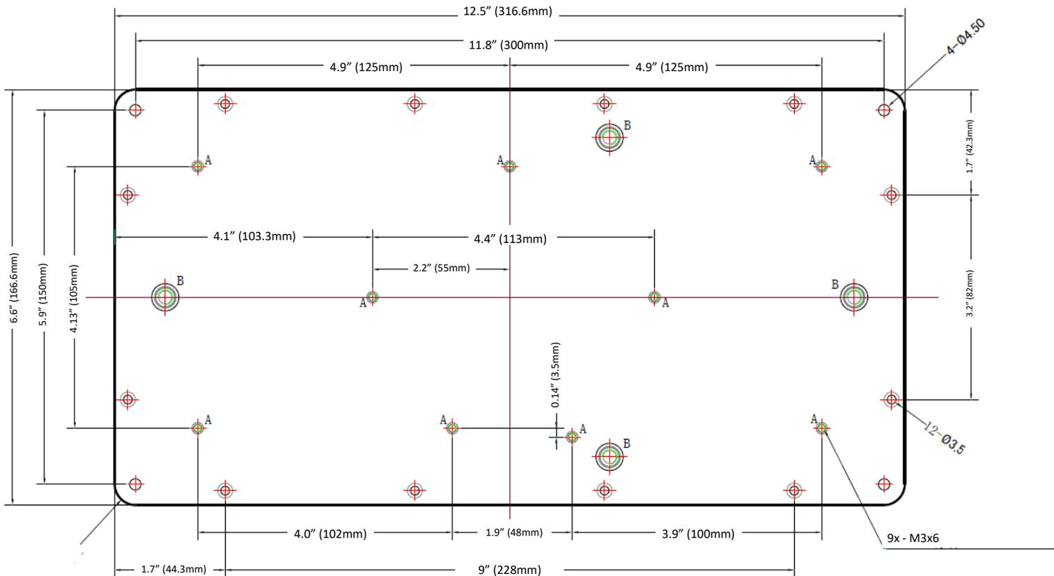
\*NOTE: The threaded inserts labeled "B" in the above graphic are 1/4"-20TPI and are meant to be used with I-beam clamps for easy mounting to the I-beams
