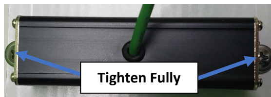
Figure 13 - Tighten Down Screws
