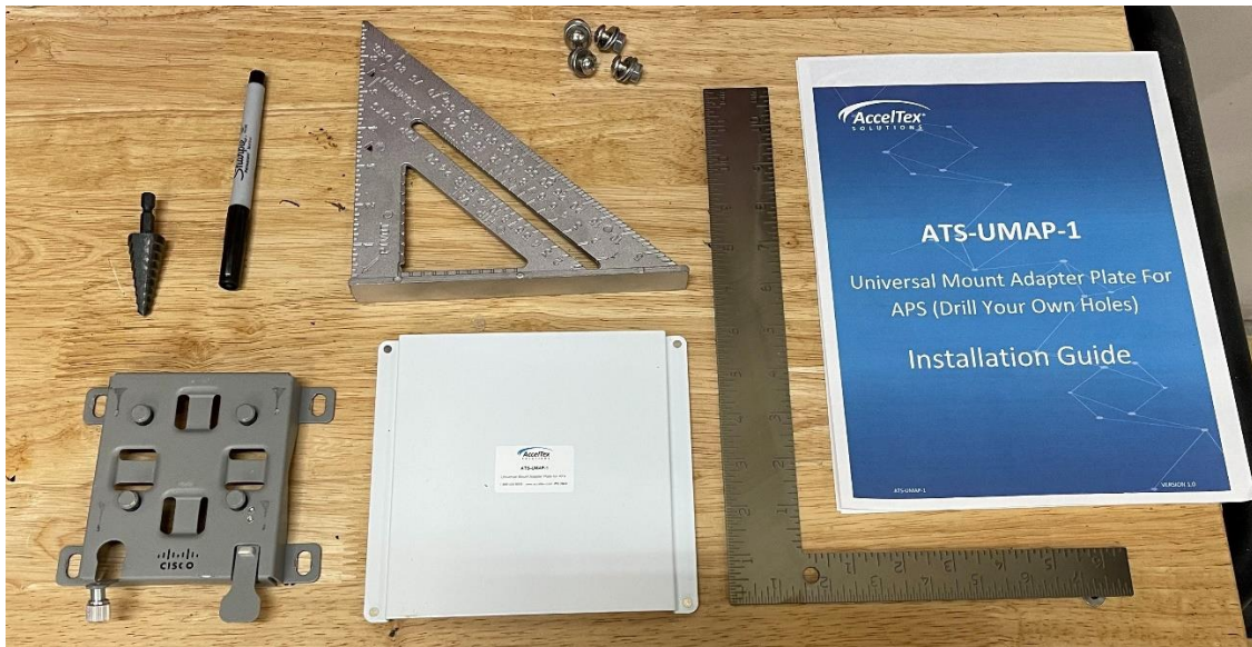
Figure 1 Example showing the set-up of an ATS-UMAP-1 for a Meraki MR72 backplate.
