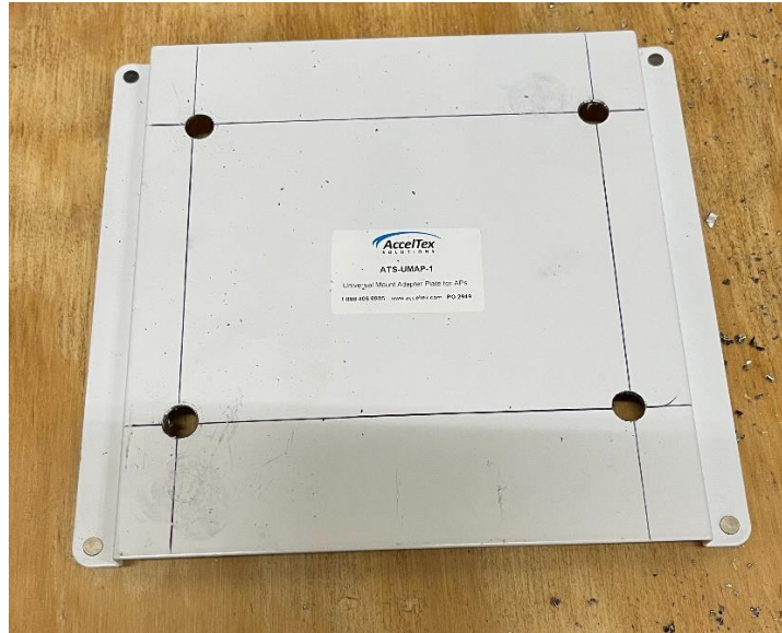
Figure 4 Hole pattern drilled with an appropriately selected bit made from carbon tool steel and oversized holes for bolt clearance.
